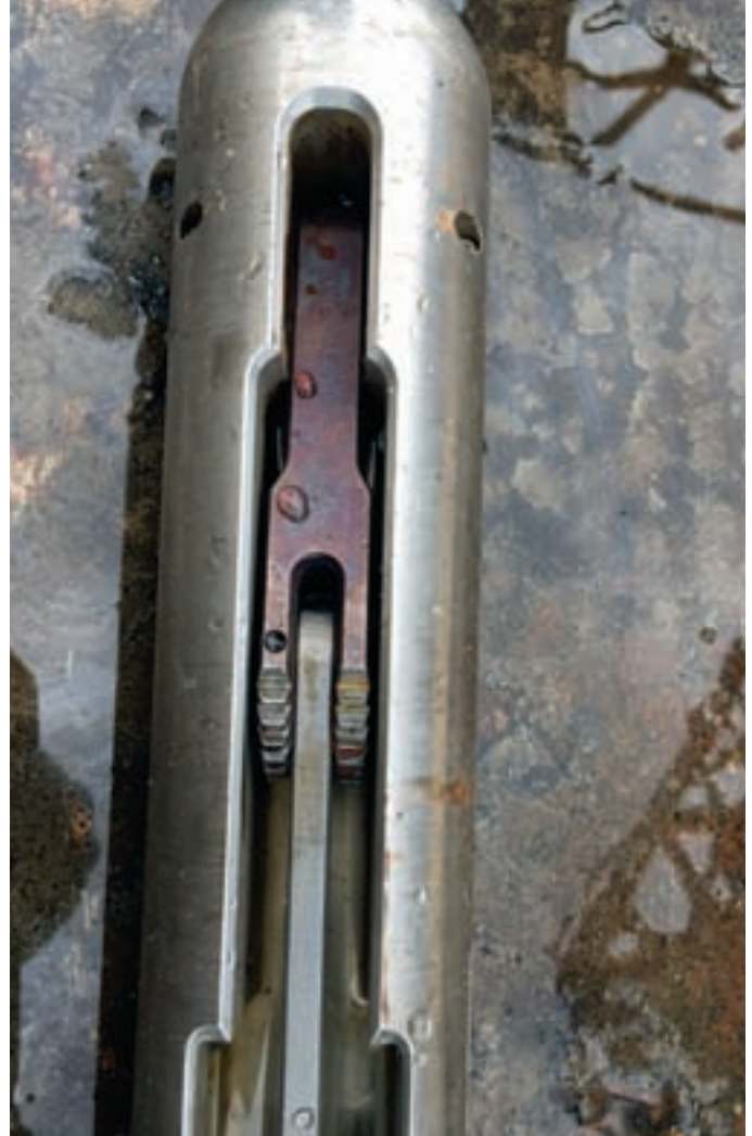
Pictured on the left is the front gripper for the Production Technology Team's compact hydraulic tractor, while on the right is the actual tracting mechanism for the new technology, which is considered a major breakthrough with global implications in small diameter extended reach wells. The technology is cost-effective, as it is rigless.
