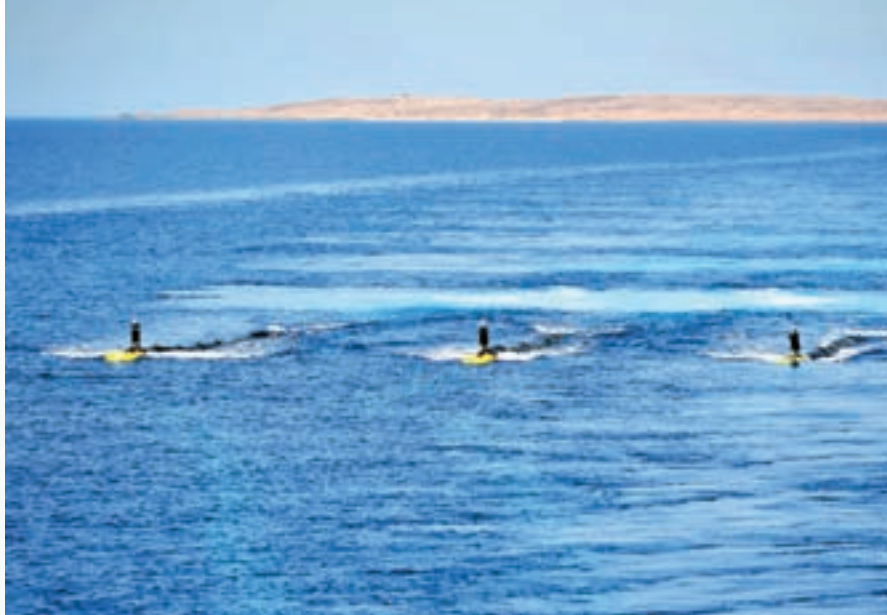
Firing every 10 seconds when in operation, the air gun shots, like those pictured here, reach an average of 5,000 shots per day. It is the acoustic waves generated by these shots that is picked up by the nodes on the sea floor, creating crucial seismic data.
