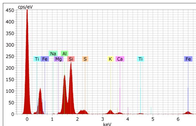
Fig. 2. EDS spectrum of the shale sample.
