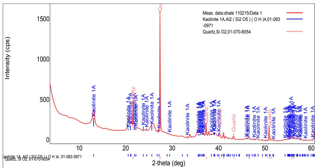
Fig. 1. XRD spectrum showing the spikes of the shale sample.
