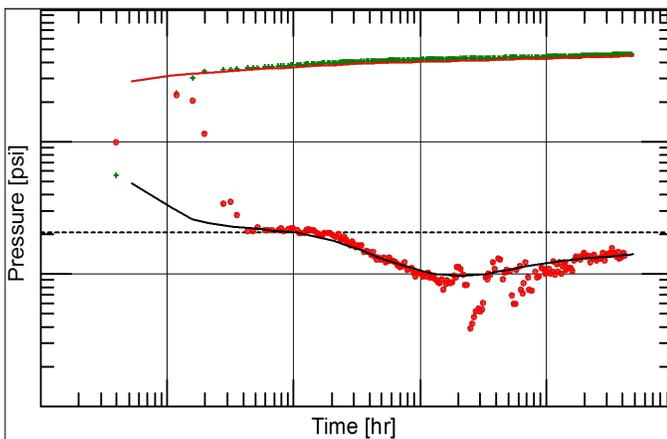
Fig. 6. Diagnostic log-log plot with match of Well-A data using a numerical solution to calibrate the fracture network.
