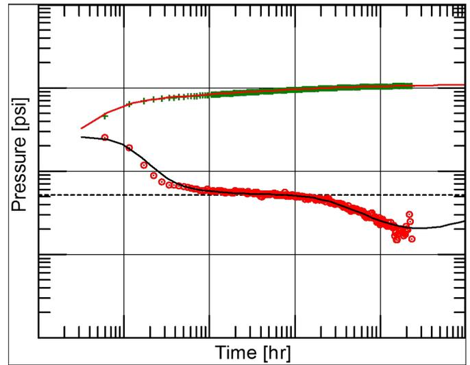
Fig. 7. Diagnostic log-log plot with match of Well-B data using a numerical solution to calibrate the fracture network.
