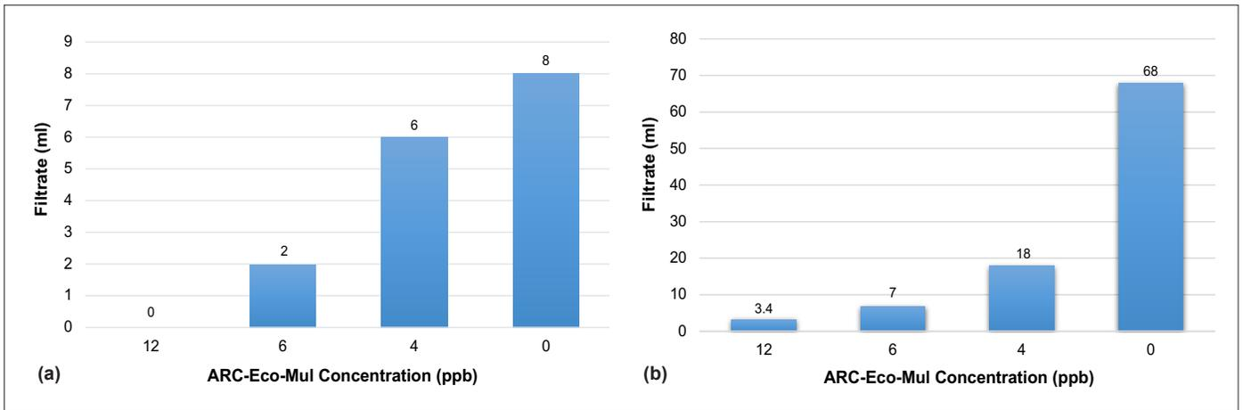
Fig. 5. HPHT spurt loss (a), and HPHT fluid loss (b).
