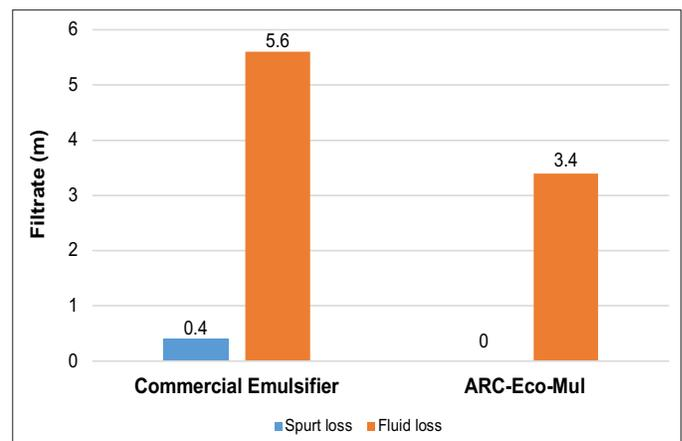
Fig. 3. HPHT spurt and fluid loss of the commercial emulsifier and ARC-Eco-Mul formulation.
