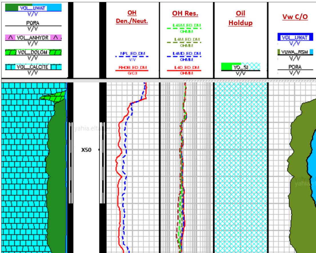
Fig. 5. An example of borehole fluid reinvasion. Track 4 is the borehole fluid holdup.
