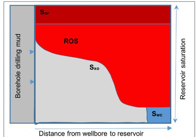
Fig. 1. Illustration of the effect of drilling mud filtrate invasion on near wellbore reservoir saturation.
