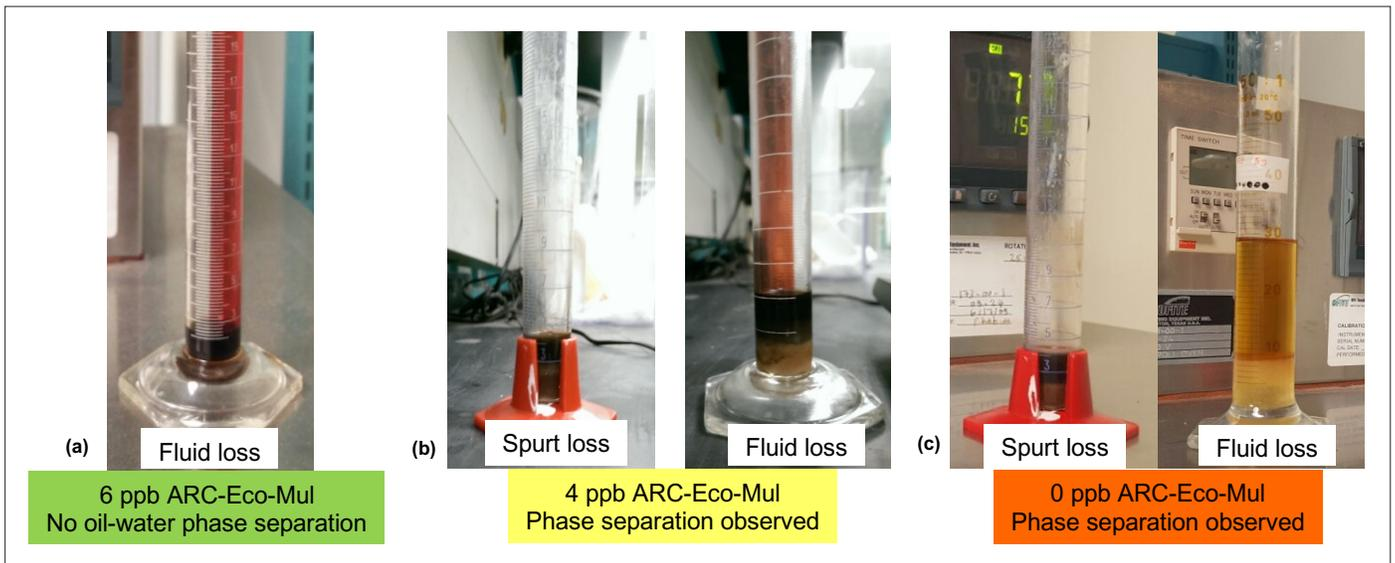
Fig. 6. Results of the HPHT fluid loss experiments of the ARC-Eco-Mul emulsion. At 6 ppb, there is no oil-water phase separation (a), at 4 ppb, phase separation is observed (b), and at 0 ppb, a distinct oil-water separation is seen (c).
