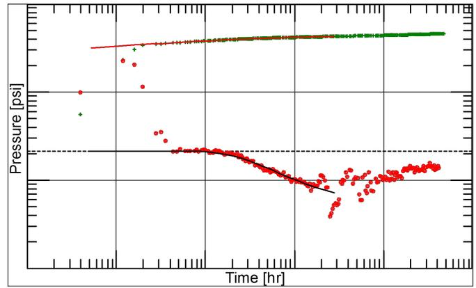
Fig. 3. Diagnostic log-log plot with a match of the data for Well-A using an analytical solution to estimate the distance to the fault.
