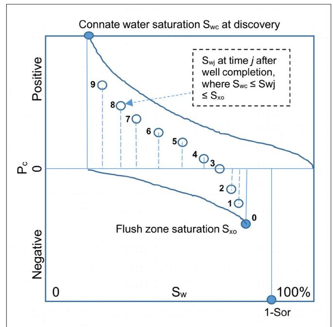
Fig. 2. Model used to explain changes in near wellbore reservoir saturation after drilling.
