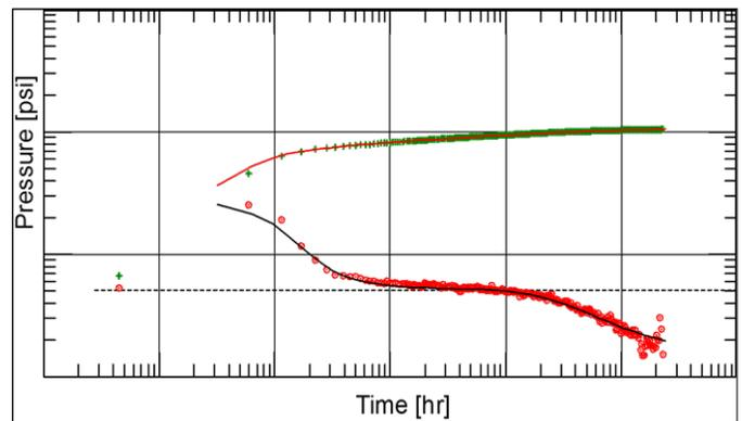
Fig. 4. Diagnostic log-log plot with a match of the data for Well-B using an analytical solution to estimate the distance to the fault.
