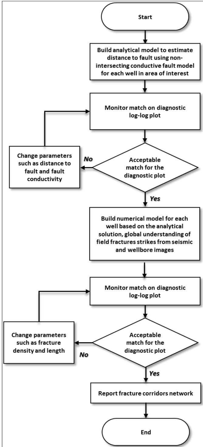
Fig. 1. Proposed workflow to characterize interwell fracture corridors.
