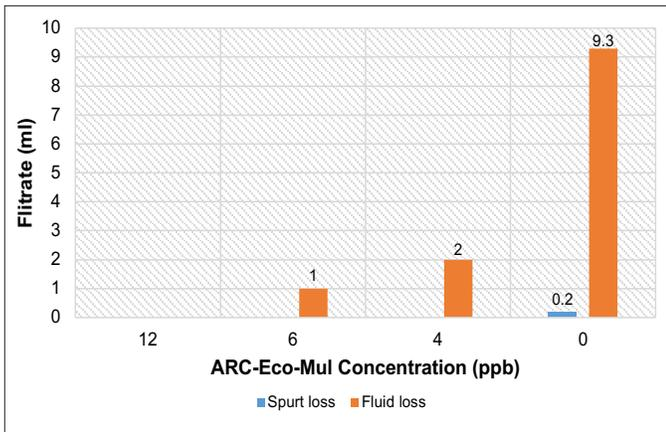
Fig. 4. Spurt and fluid loss for the API filtration control properties of the ARC-Eco-Mul.
