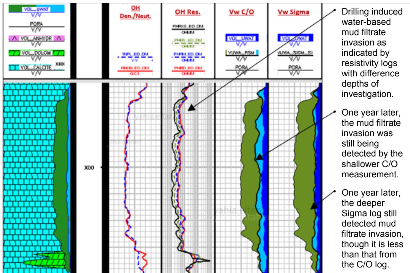
Fig. 3. An example of drilling mud filtrate invasion and its effect on time-lapse PN logging. Tracks 4 and 5 display C/O and Sigma log results (dark blue is water volume (Vw) derived from a deep open hole resistivity log, light blue is Vw from a PN log, and green is oil).
