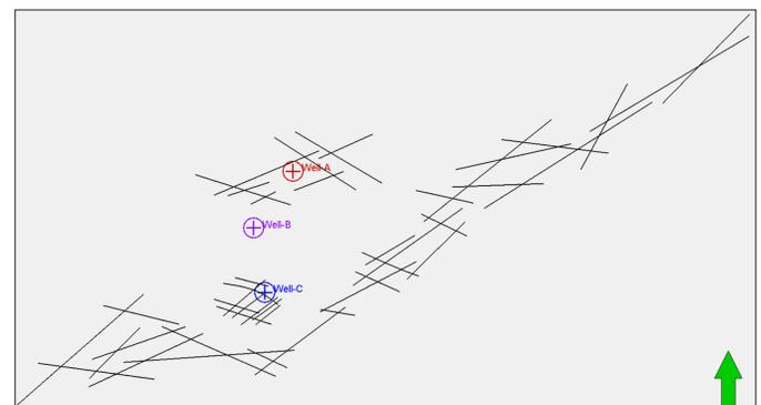
Fig. 9. Fracture corridors in the area of interest calibrated with analytical and numerical models using well test data from Wells A, B, and C.
