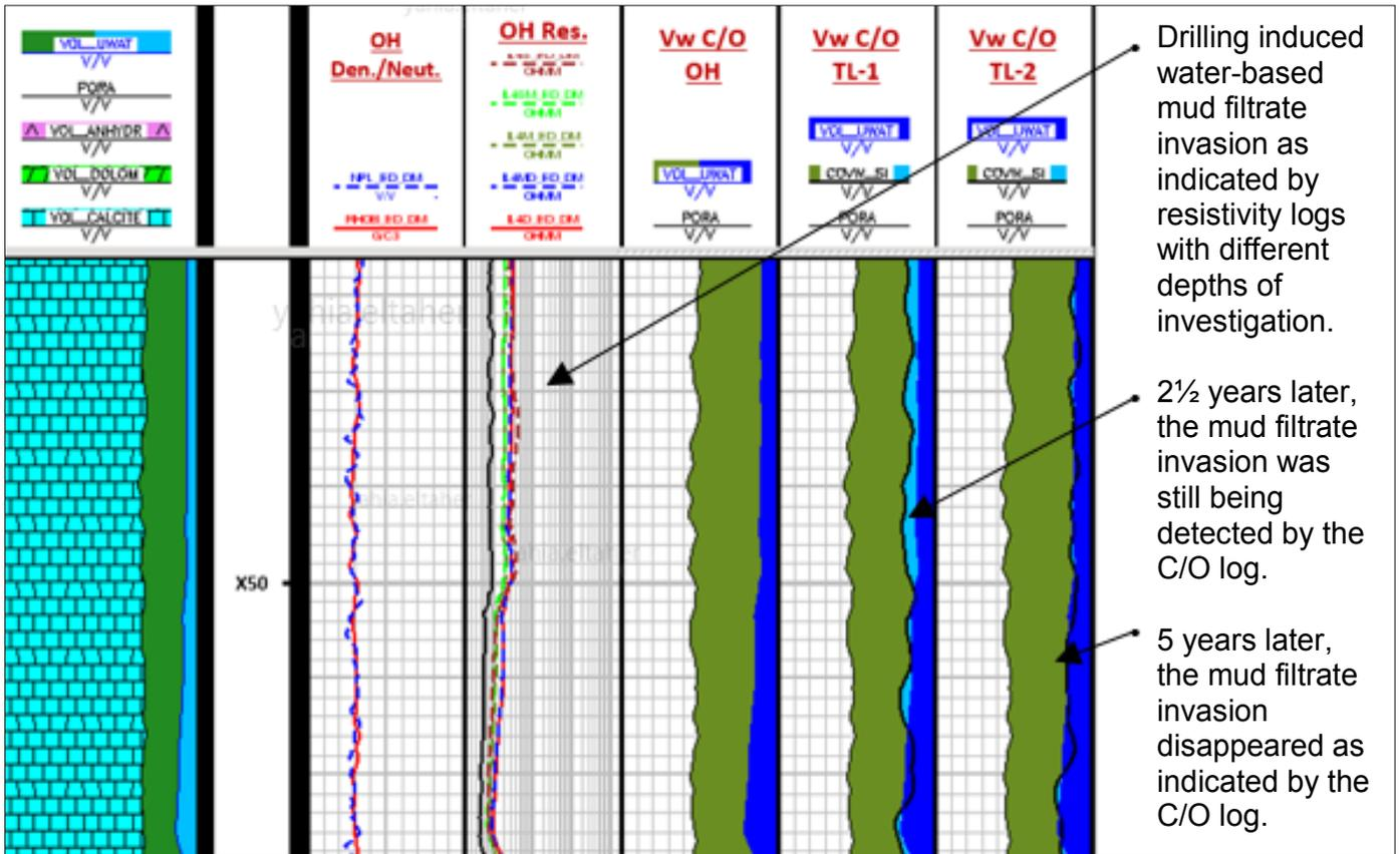
Fig. 4. An example illustrates dissipation of mud filtrate invasion in this observation well completed cased hole. Tracks 5 and 6 are time-lapse C/O logs run 2½ and 5 years after drilling, respectively.
