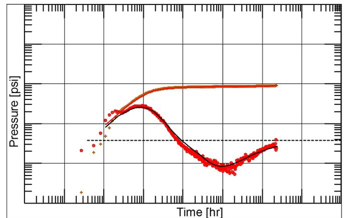
Fig. 8. Diagnostic log-log plot with match of Well-C data using a numerical solution to calibrate the fracture network.
