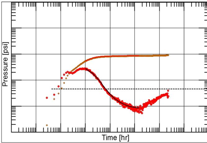
Fig. 5. Diagnostic log-log plot with a match of the data for Well-C using an analytical solution to estimate the distance to the fault.
