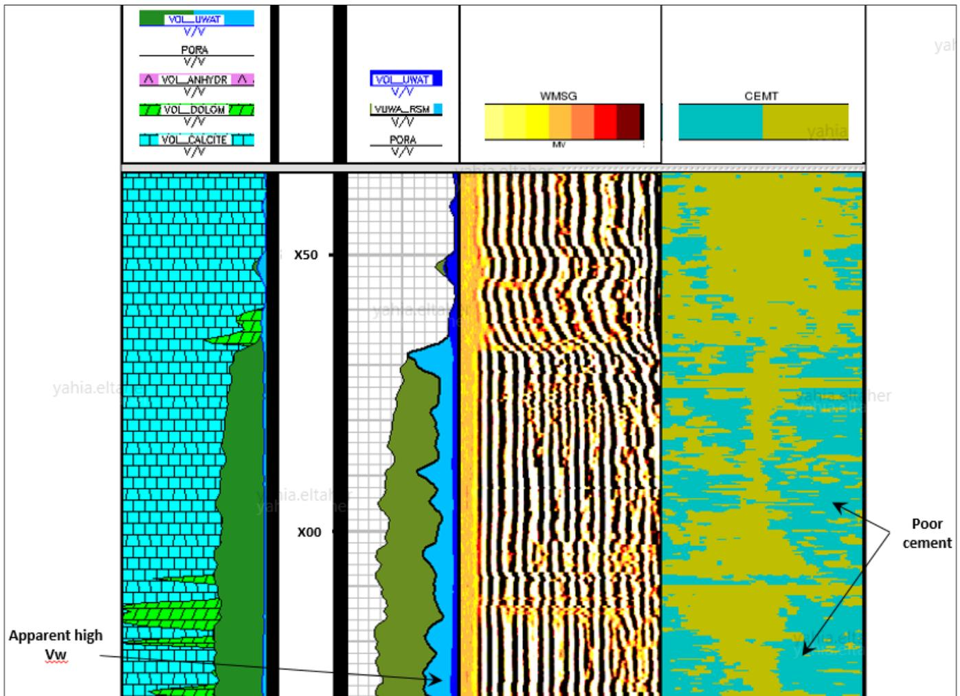
Fig. 6. Effect of poor cement quality on apparent water saturation calculated from C/O measurements.
